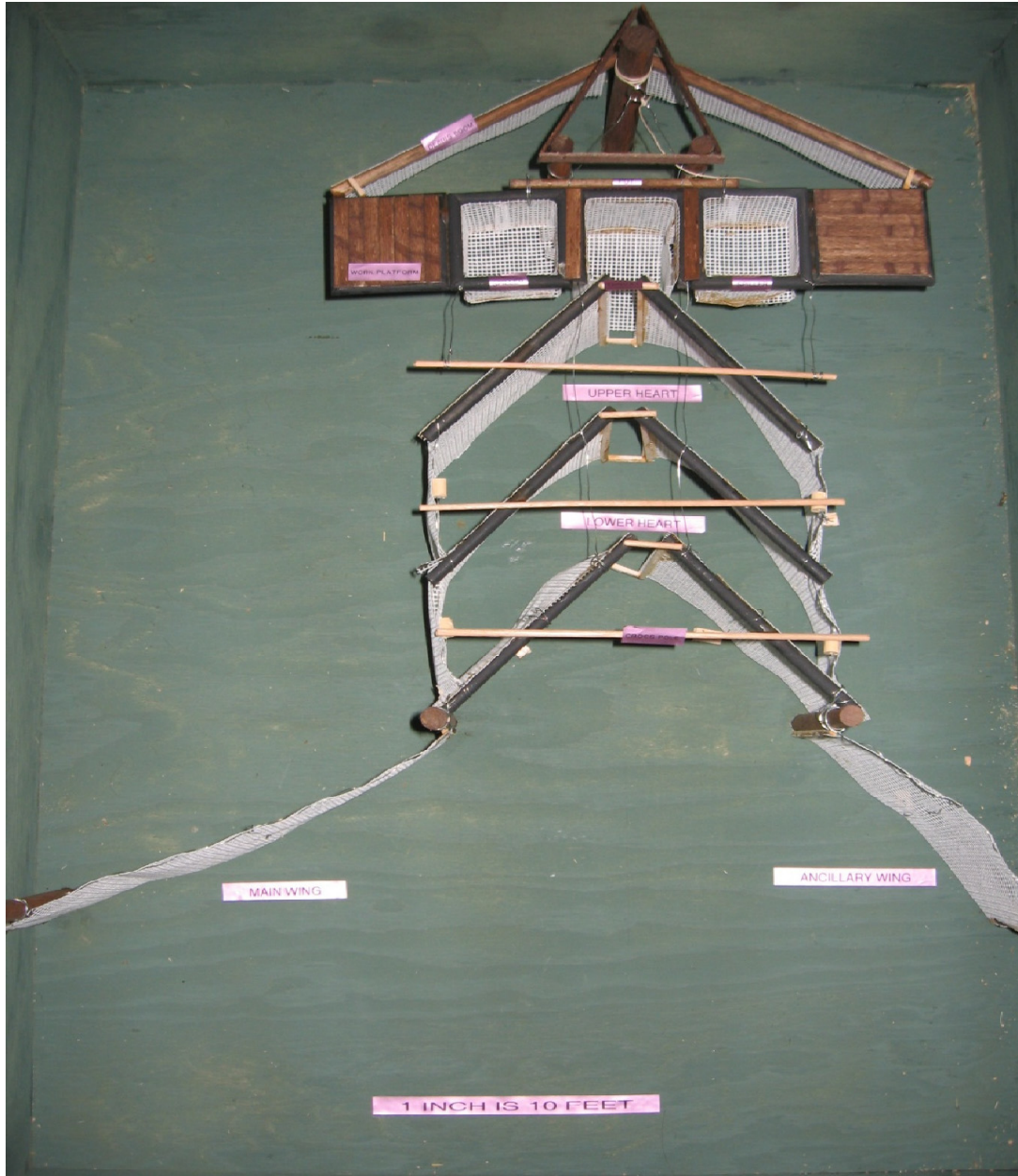
Figure B-5. Model of proposed Colville floating fish trap (modified Alaskan trap).
