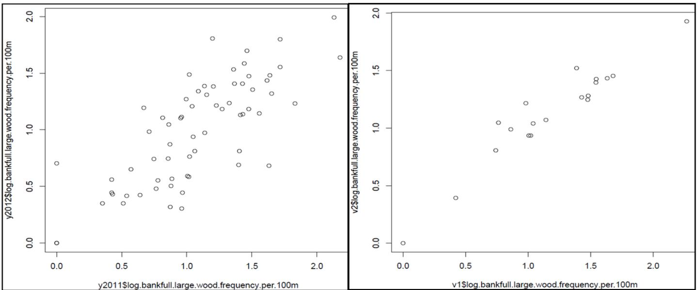
**Figure 16.** The relative magnitude of the interaction vs. residual variance component for the metric 'bankfull large wood frequency' is high, implying that there should be a noisier relationship in the 2011 vs. 2012 plots compared with the visit 1 vs. visit 2 plots, as illustrated by this pair of plots.
