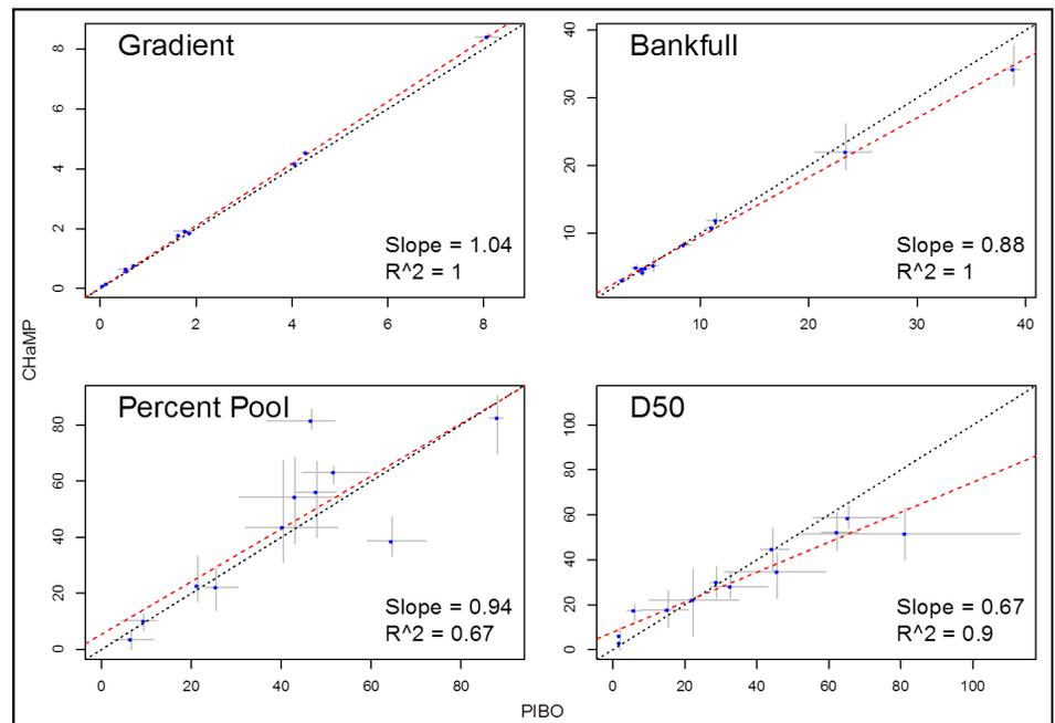
**Figure 1. Examples of CHaMP and PIBO attributes evaluated during the 2012 protocol comparison study that were measured the same way or could be transformed between programs based on strong relationships.**
