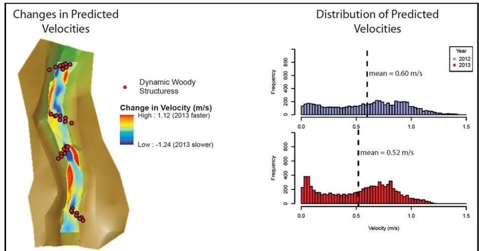
**Figure 25. The difference in water velocities pre-treatment (Before) and post-treatment (creation of pools via wood additions) in a reach of the South Fork of the Asotin.** Velocity (Before) is subtracted from velocity (After) to create another surface.
