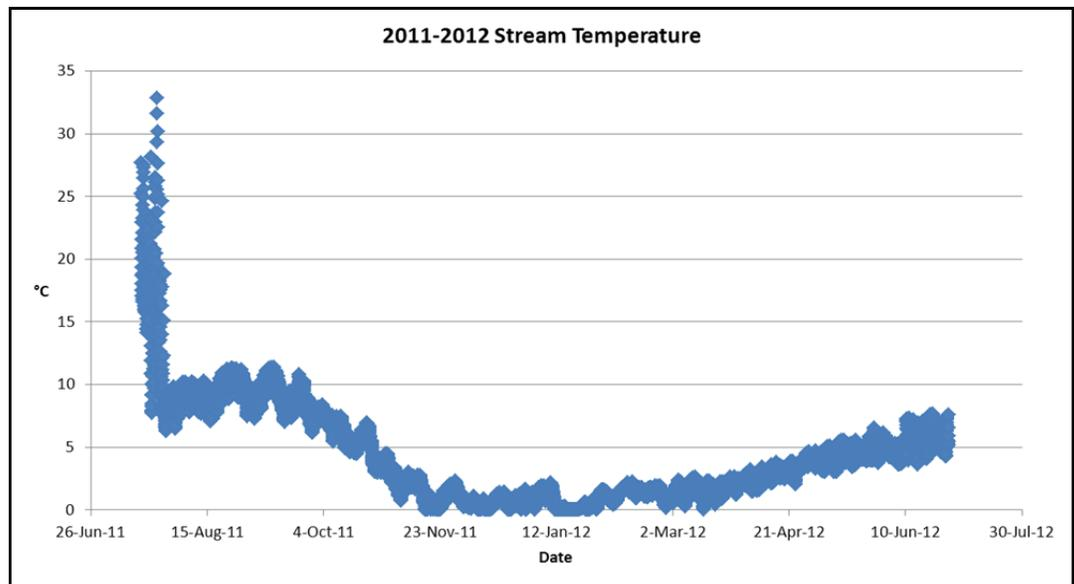
**Figure 34. A typical temperature profile graph for a CHaMP site in the Wenatchee River watershed that includes a week of leading air temperature readings.**
