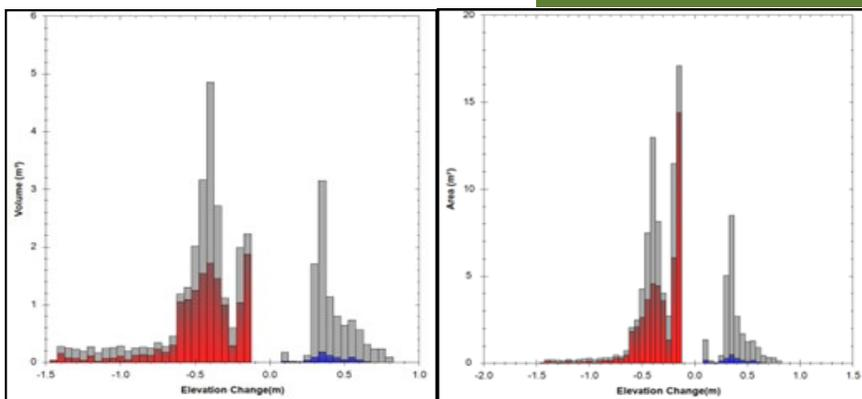
**Figure 36. In 2012, GCD between visits of the same site was added to the RBT. The change detection isolates the differences in the topographic survey and removes the portion of the change that is uncertain (either because the change was too small or because there was an error with one of the surveys). The GCD analysis outputs the area and volume of change, as well as segmenting this change into erosion, deposition, by tier1 and tier 2 channel units, inside and outside the channel.**
