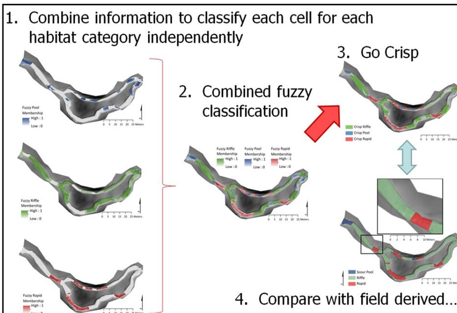
Figure 28. Using the RBT and many lines of evidence to derive fuzzy habitat units
