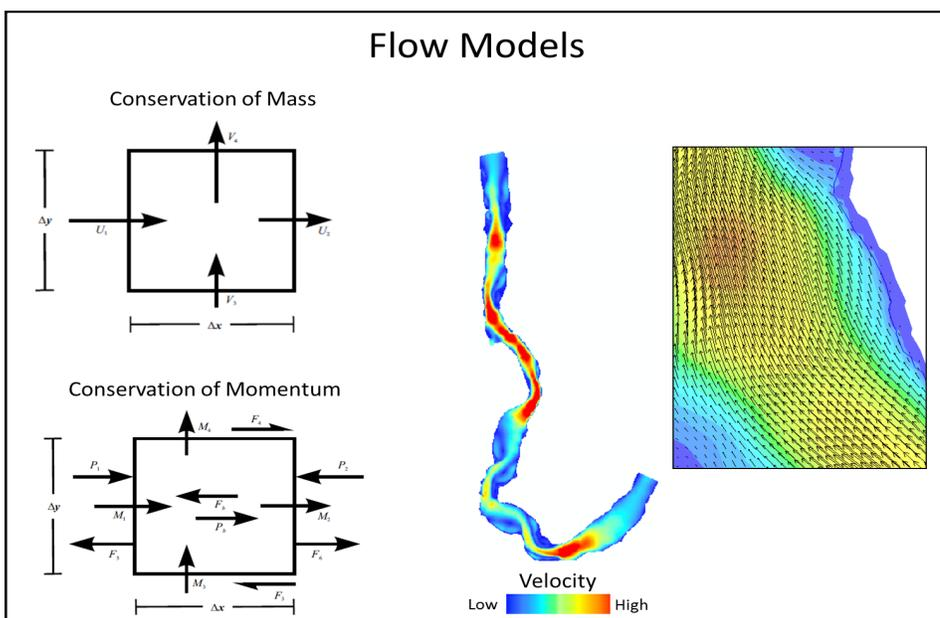
Figure 30. Example of hydraulic model computational mesh and graphical output.
