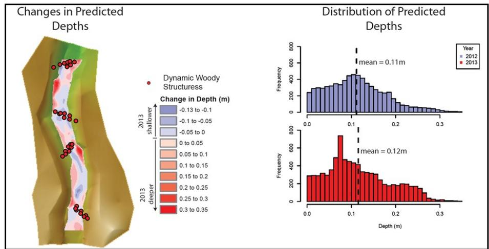
**Figure 24. The difference in water depths pre-treatment (Before) and post-treatment (creation of pools via wood additions) in a reach of the South Fork of the Asotin.** If depth (Before) is subtracted from depth (After) for each pixel that has an XY coordinate, another surface is created that spatially describes the change in depth of the reach due to restoration.
